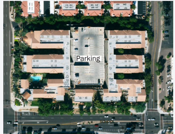
ENCOURAGED - Locate at- and above-grade parking facilities at the rear or interior portions of a site.
