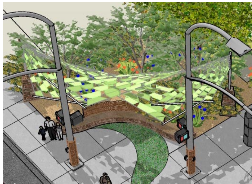
Dry laid sandstone pier with trapezoid shape low walls and metal seat back panels at primary Green Spot
