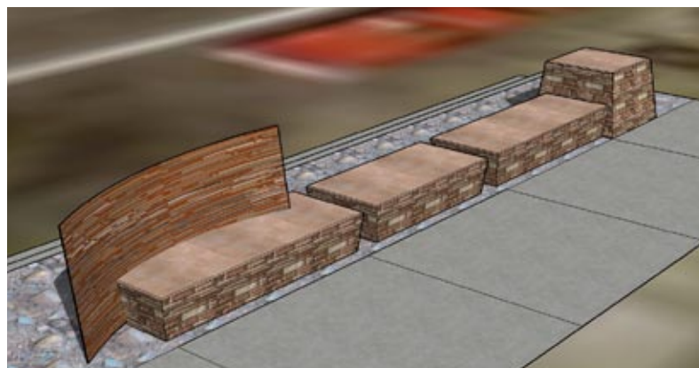
Low seat walls will be made out of materials specific to the segment, yet will look continuous in form throughout the corridor
